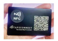
Note: The NFC Tag is embedded in a recess in the card, it cannot be moved or rotated.
